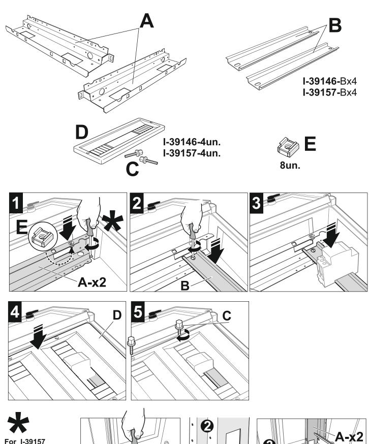
For I-39157 use before 4xplastic elevator pieces (included with the enclosure)
